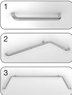
MAAX Outlook *plus* textured stainless steel grab bars feature an easy to clean smooth surface. Straight<sup>1</sup>, L-shaped<sup>2</sup> or U-shaped<sup>3</sup>, in multiple dimensions. There is one for every need. All grab bars are 1 ¼" in diameter, securely bolted through the wall, and are designed and tested to withstand up to **300 lb** of pressure as per major accessibility building codes.
